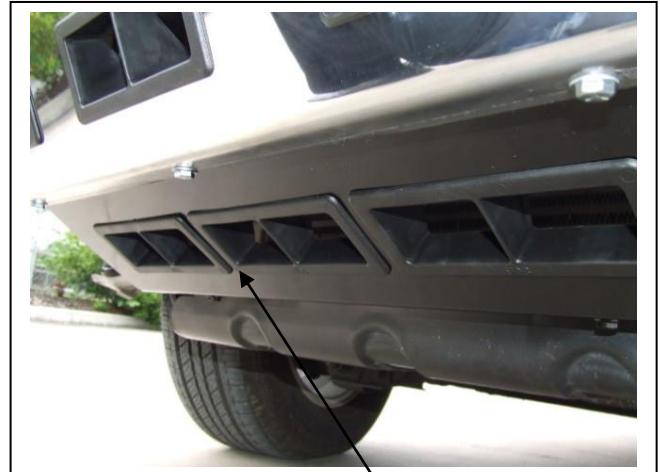
Figure 12: Under body Alloy Bash plate, with 3mm air vents fitted, ECB logo to bottom
